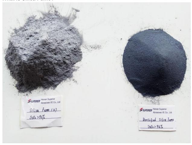
Silica fume, also known as volatilized silica, micro silica, or condensed silica fume, is a pozzolanic material, which presents a gray-colored d powder, somewhat similar in appearance to fly ashes or Portland cement. It consists primarily of non-crystalline (or amorphous) Silicon Dioxide (SiO2), with each particle being approximately 0.01 times the size of an average cement particle.
